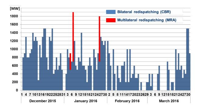
The result of such frequent usage (and at such high level) for CBR is a rapid increase of energy volume necessary to realise these remedial actions what is shown on the figure below (without energy activated within DC Loop Flow). There was more than 330% increase of mentioned volume, when comparing winter 2015/2016 to winter 2014/2015:
